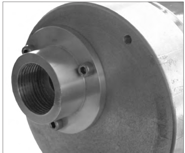
Fig. 9. Mounting the C7061F1xxx detector
